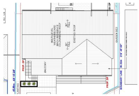
The proposal consists of new hip roof over the existing house towards the rear side of the house. The roof material will me metal colourbond roof which will be held by timber beams and rafters with timber posts to support the proposed roof. (Refer to the architectural plan for more information).
