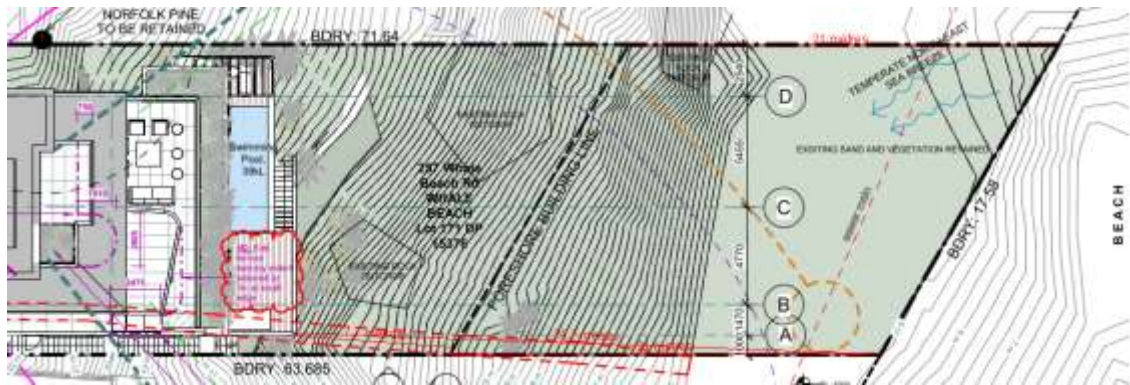
Figure 2. Rear section of the proposed development demonstrating the Foreshore Building Line (FBL) and the distance of FBL from the rear boundary (21m), the distance of the development from the rear boundary 28.7m and the distance of the development behind the FBL (7.7m).
