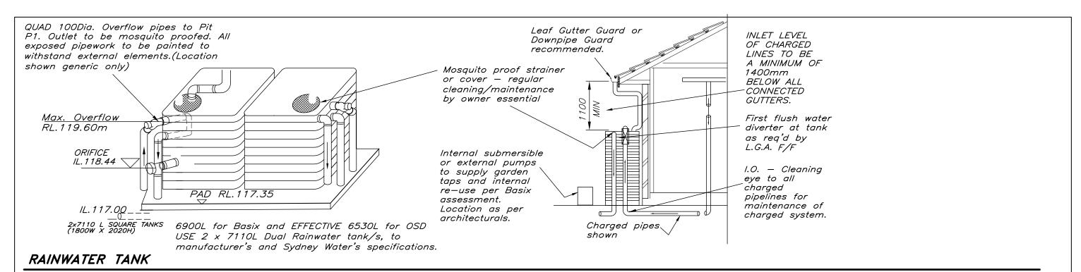
TANK DETAILS SHOWN ARE A SUGGESTED CONFIGURATION ONLY. ANY MODIFICATIONS TO TANK VOLUME OR INLET AND OUTLET LEVELS MUST BE APPROVED BY ENGINEER PRIOR TO COMMENCEMENT OF CONSTRUCTION. TANK SHAPE, & DEVICES SHOWN ARE DIAGRAMMATIC ONLY. MINIMUM OF 450 CLEARANCE (UNLESS L.G.A. REQUIRES LARGER SETBACK) TO SIDE BOUNDARIES MUST BE MAINTAINED. CLIENT IS RESPONSIBLE TO ENSURE COMPLIANCE WITH THIS IN THE INSTALLED STATE. Charged stormwater lines from Roof Areas ONLY to rainwater tank.
