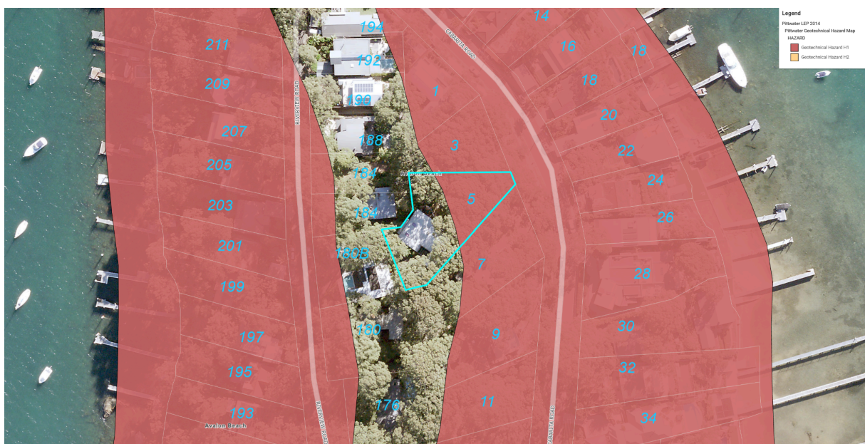
Figure 10: Geotechnical Hazard Map - site of proposal in detail (source: Pittwater Council LEP 2014)
