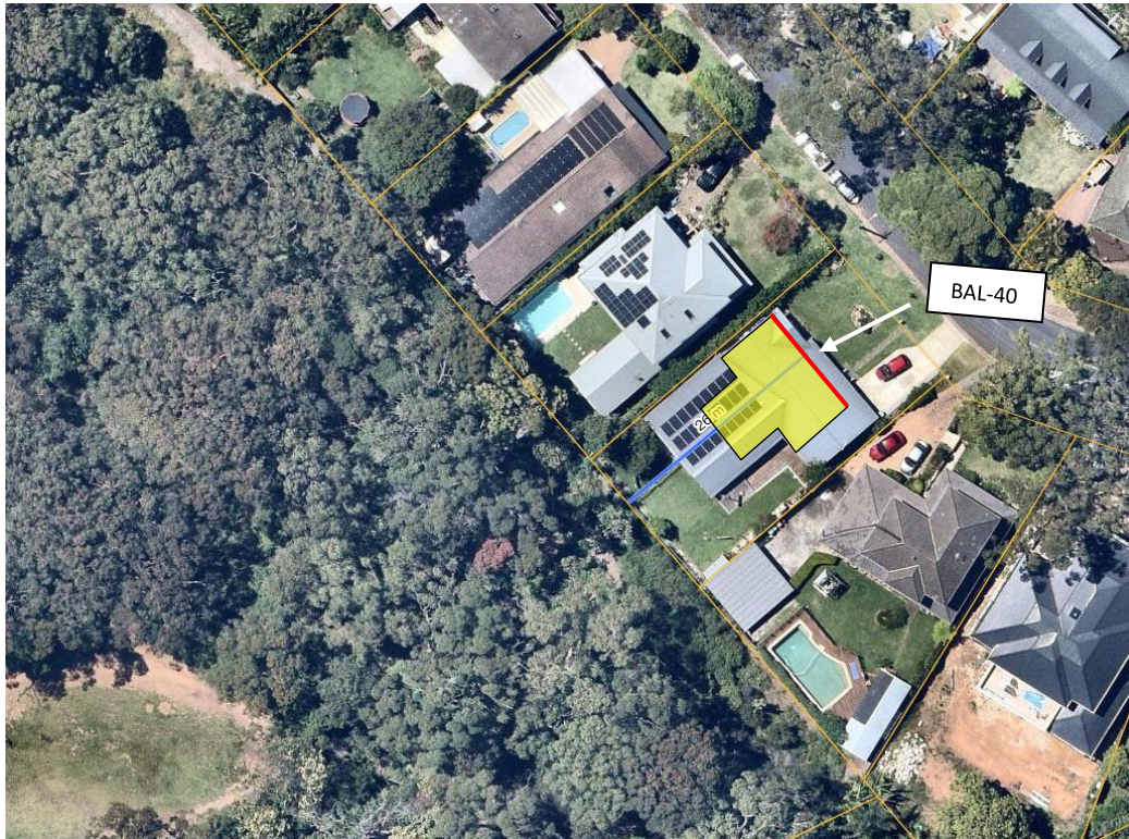
Figure 10: Site plan showing the eastern elevation that can be reduced to BAL-40.
