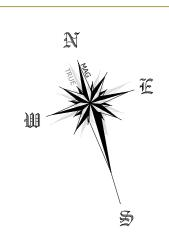
BEARINGS SHOWN HAVE BEEN DETERMINED FROM NSW LAND REGISTRY SERVICES PLANS AND ARE RELATED TO MAGNETIC NORTH. TRUE NORTH IS APPROXIMATE ONLY AND FURTHER INVESTIGATION WOULD BE REQUIRED TO DETERMINE ACCURATE TRUE NORTH.
