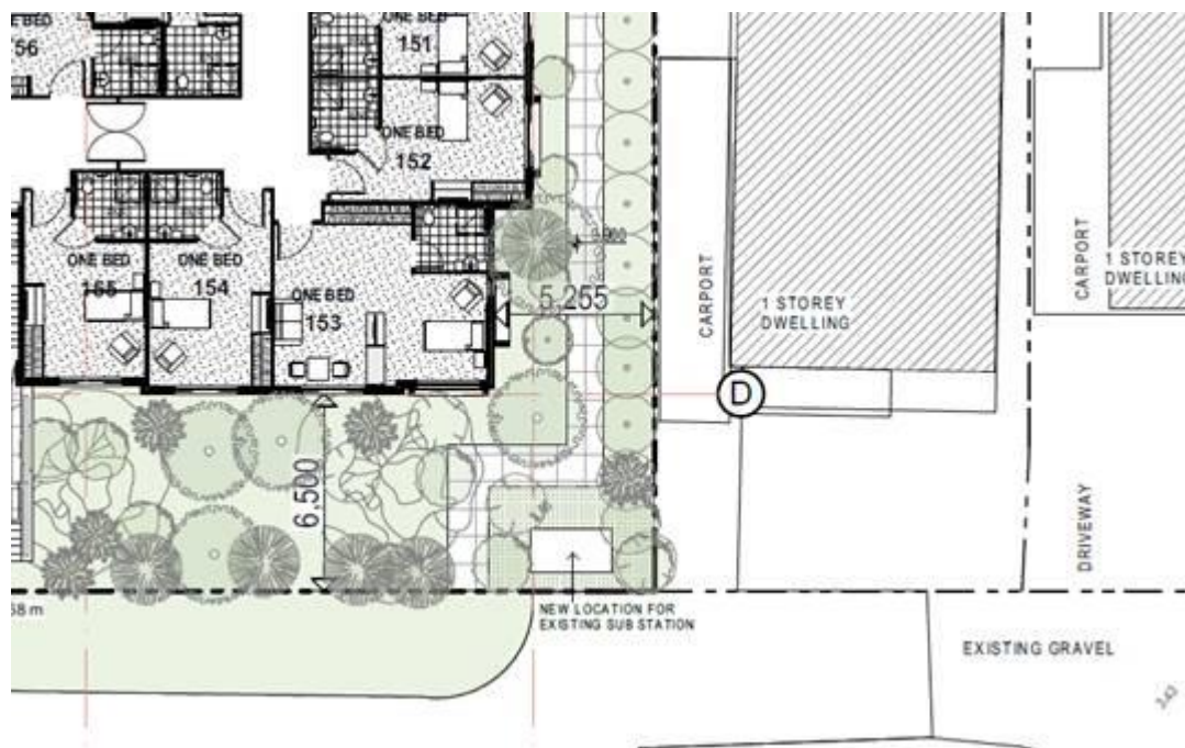
Figure 4 – Extract from site plan showing proposed location of electricity kiosk
