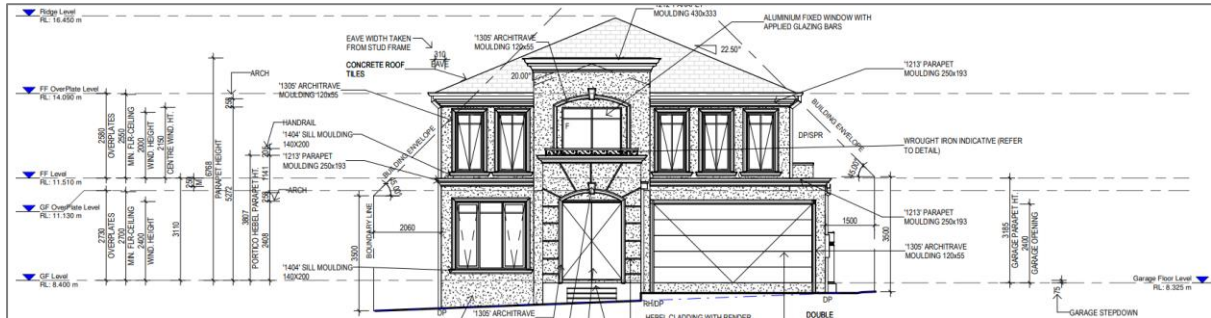
Figure 3: Front Elevation of Proposed Dwelling House
