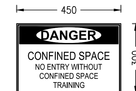
DETAIL 9 CONFINED SPACE SIGN SCALE 1:10
