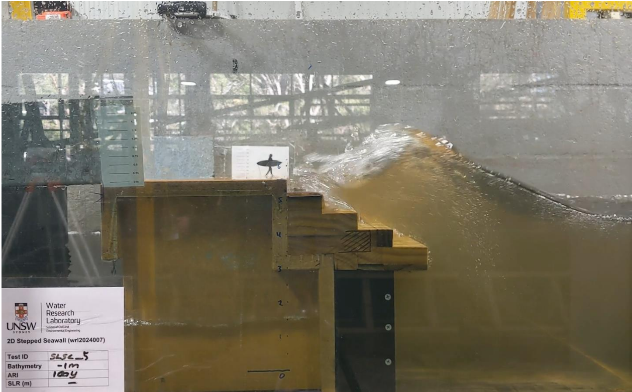
Figure 2-7 Peak wave overtopping of the promenade in the 100-year ARI storm for an eroded beach profile under present day water level conditions, with a bleacher profile seaward of the promenade.
