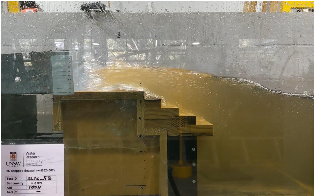
Figure 2-8 Peak wave overtopping of the promenade in the 100-year ARI storm for an eroded beach profile in 2084 after sea level rise, with a bleacher profile seaward of the promenade.
