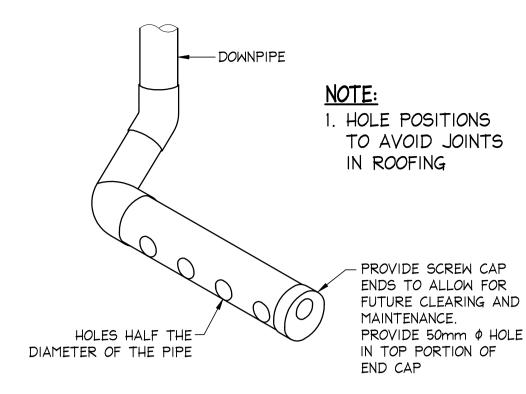
SPREADER PIPE 'SPI' DETAIL
