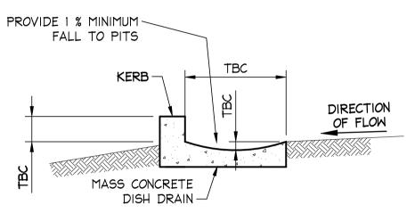
TYPICAL CONCRETE SWALE WITH KERB
