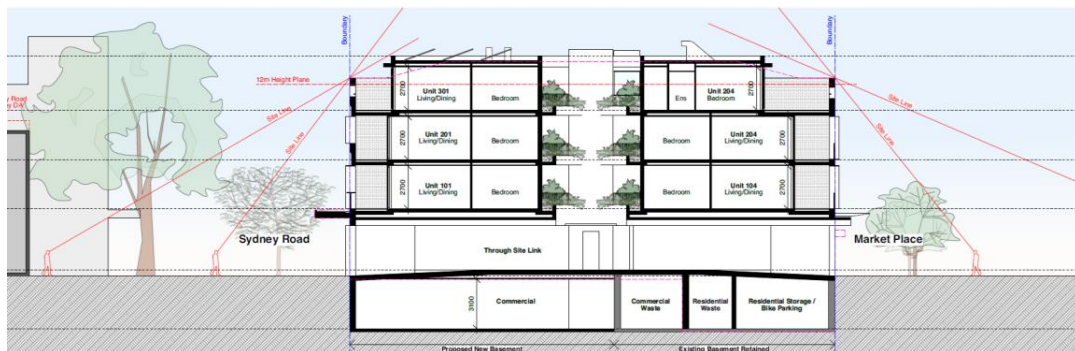
Figure 3 – Extract of Section AA with sight lines
