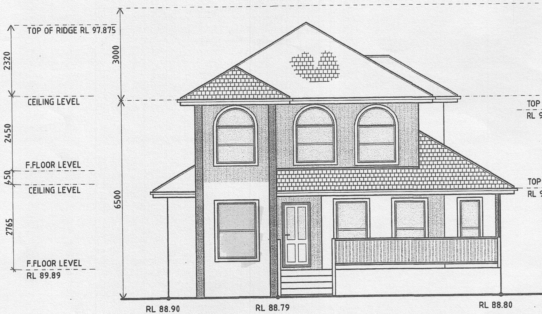
EAST ELEVATION SCALE 1:100
