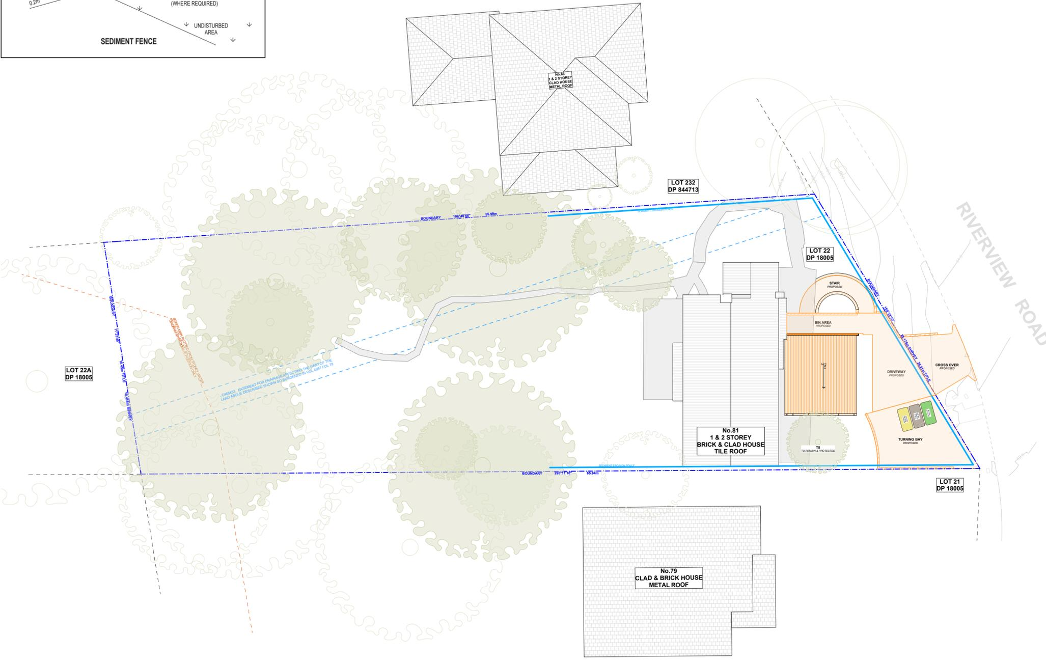
**NOTE: SITE BOUNDARY IS TO BE IDENTIFIED BY A REGISTERED SURVEYOR AND CLEARLY MARKED ON SITE PRIOR TO COMMENCEMENT OF ANY CONSTRUCTION WORKS.**
