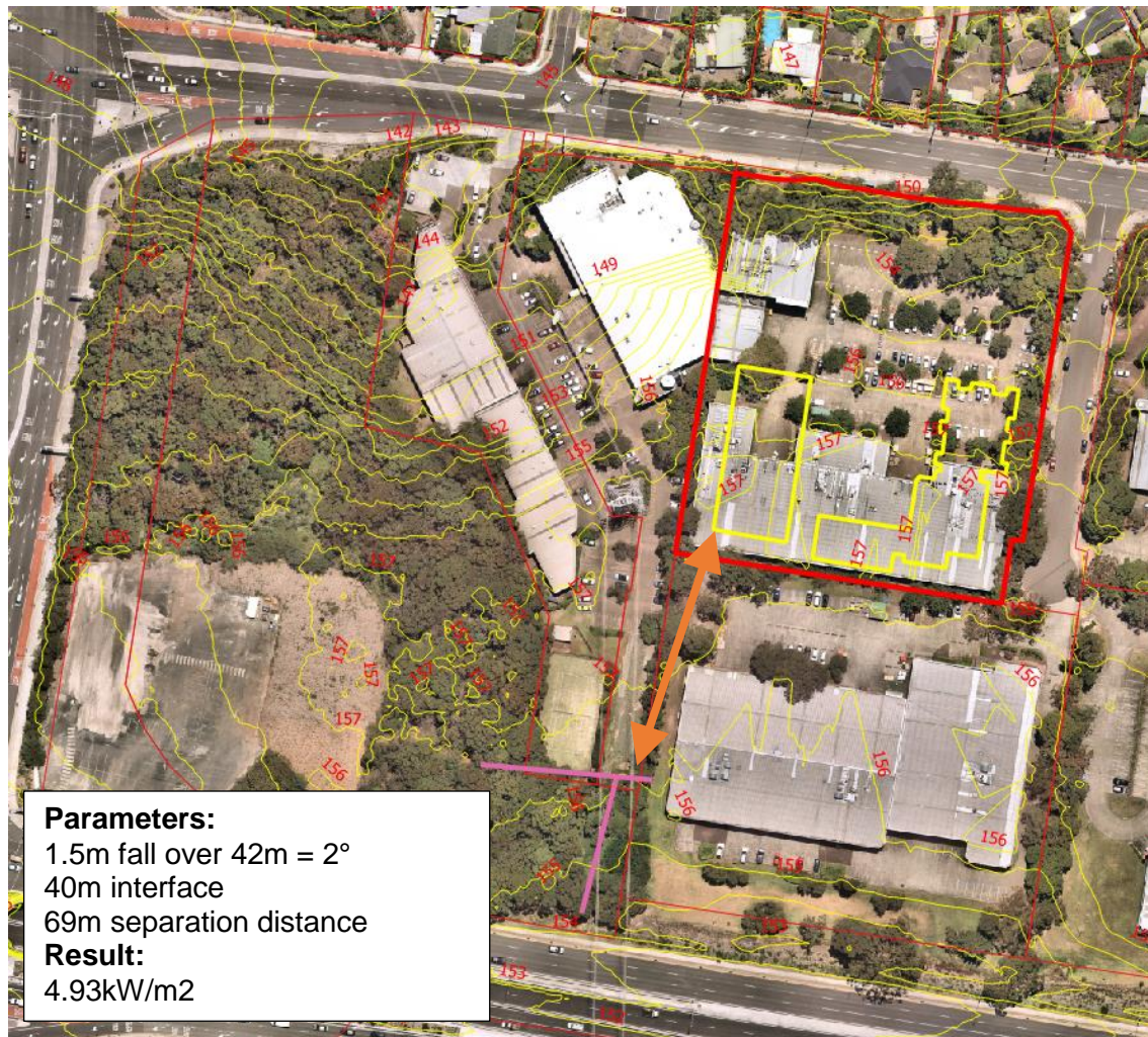
Figure 09: Aerial view of the subject area, 1 metre contours and Transect 4 Subject site (thick red outline) and proposed building envelope (yellow outline)
