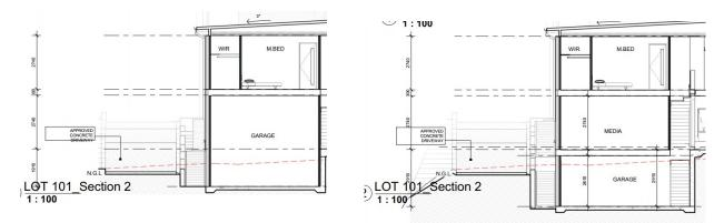
The Proposal has reduced the Driveway gradient from 24% to 15% and has made more use of space efficiently.
