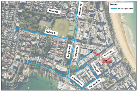
Figure 5.2: Proposed truck route (Inbound trucks up to 8.8m MRV)
