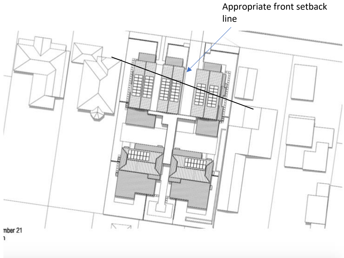
Plan view from Shadow Diagrams report showing bulk and scale of the development in comparison to neighbouring properties (north is towards the top of the diagram). The black line shows the front building line to maintain appropriate setback with the adjacent houses (not carports or outbuildings).
