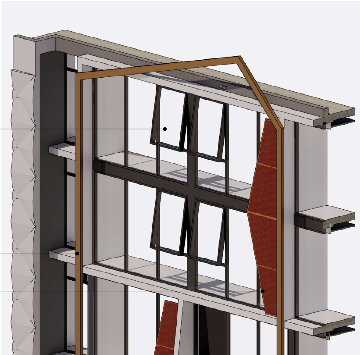
FEATURE OPERABLE WINDOW: SECTIONAL PERSPECTIVE
