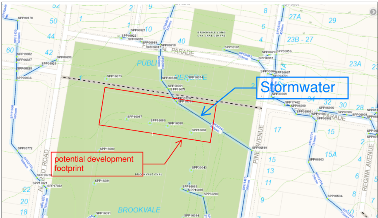
Figure 8 Existing Stormwater Layout
