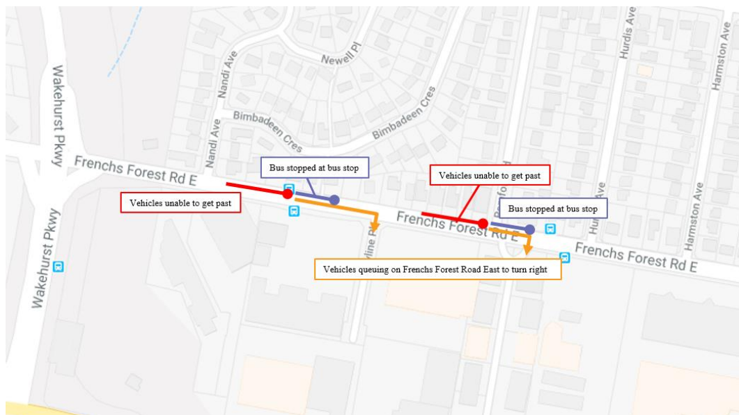
Figure 19: Bus stops on Frenchs Forest Road East
