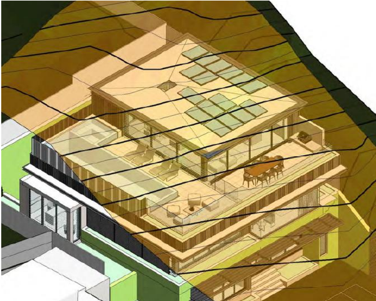
Figure 11: Plan extract showing 8 metre building height blanket (in yellow) determined from assumed undisturbed levels on the site being the ground level (existing) of the land prior to any development occurring with the building height breaching elements shown in yellow.
