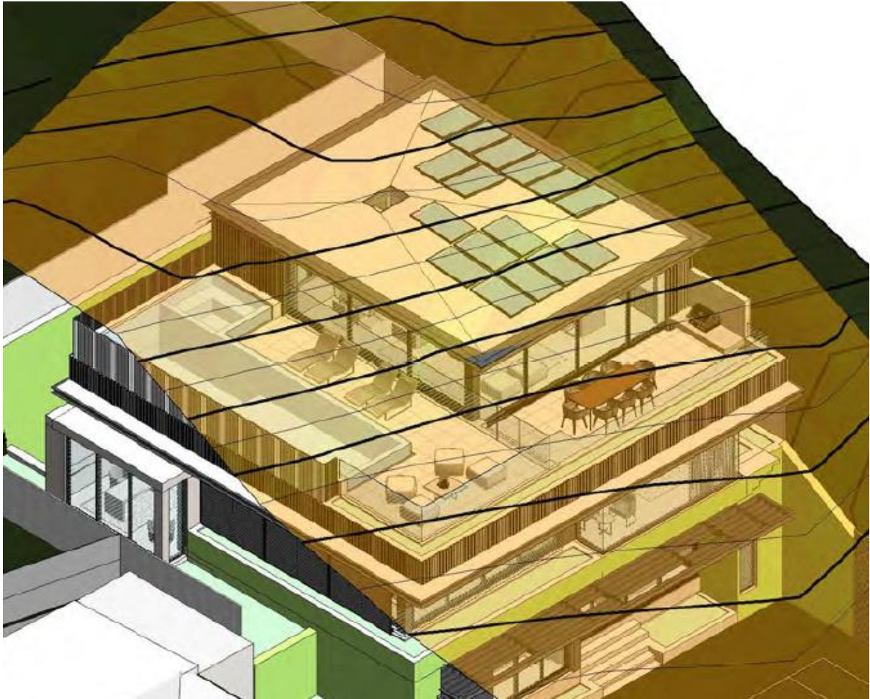
Figure 5: Plan extract showing 8 metre building height blanket (in yellow blue) determined from assumed undisturbed levels on the site being the ground level (existing) of the land prior to any development occurring with the building height breaching elements shown in grey.
