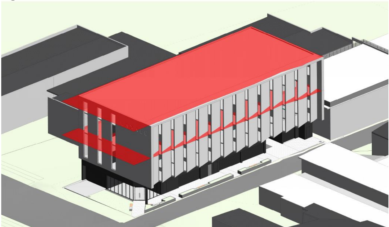
Figure 2 - Building height breaching elements showing the 11m and 18m building height planes
