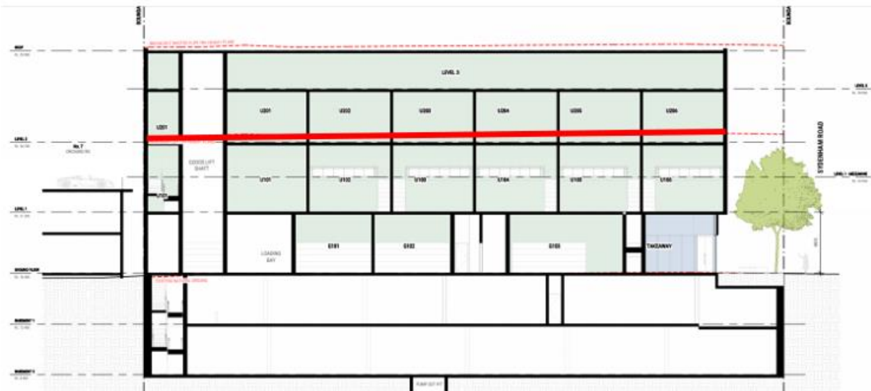
Figure 1 - Plan extract showing extent of building height breach with the red line showing the 11 metre height standard measured above ground level (existing)
