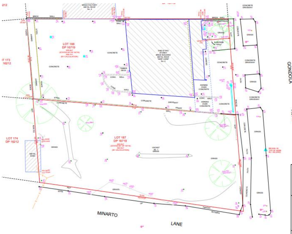
Figure 1 – Extract of site survey
