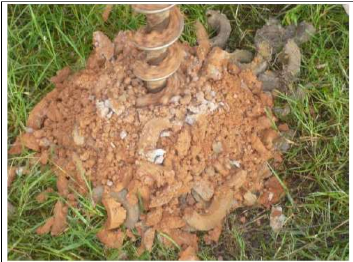
Figure 4.3 – Typical Orange Coloured Clay Turnings at Borehole MW1
