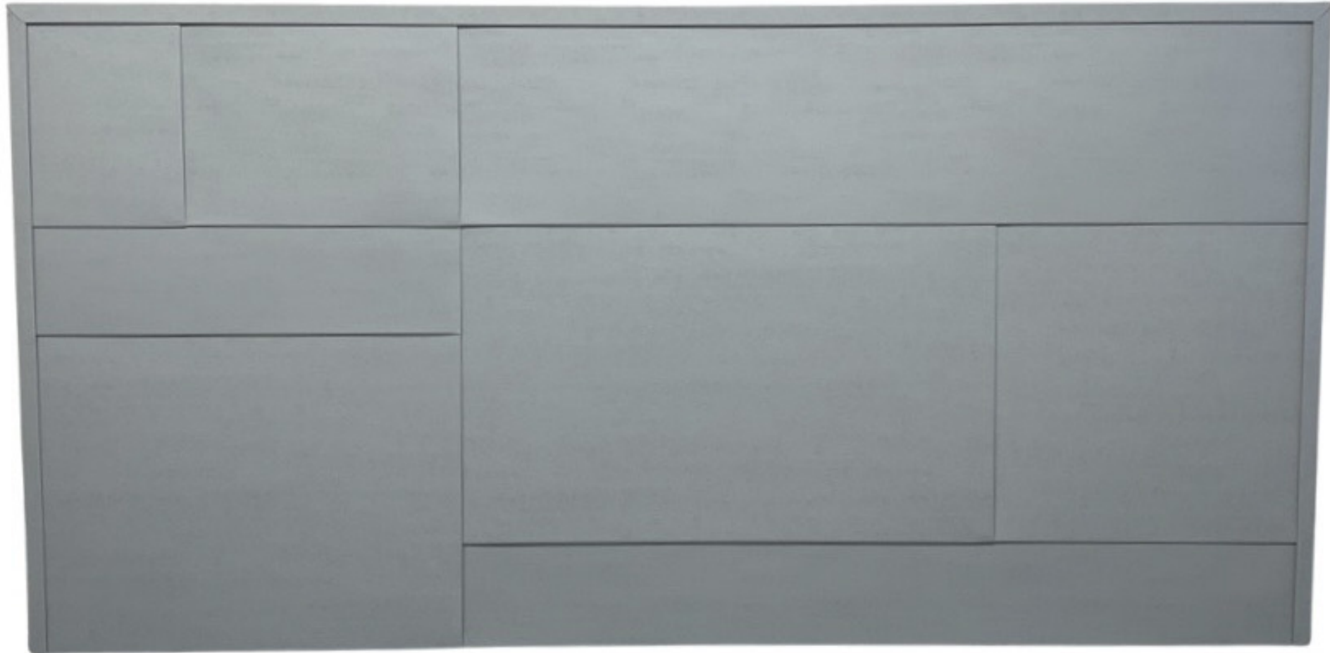
SECTION 4.55 APPLICATION AMENDMENT - SHOWN CLOUDED IN RED: FF'S FACADE UPDATED FLATLOCK ALUMINIUM CLADDING - GREY COLOUR - MATT FINISH
