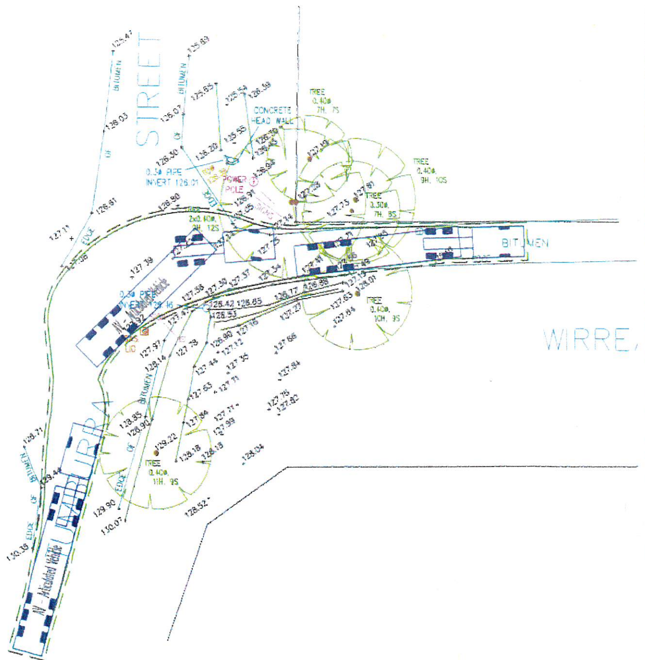
19m Semi "Float" Truck Right-Turn Turning Path
