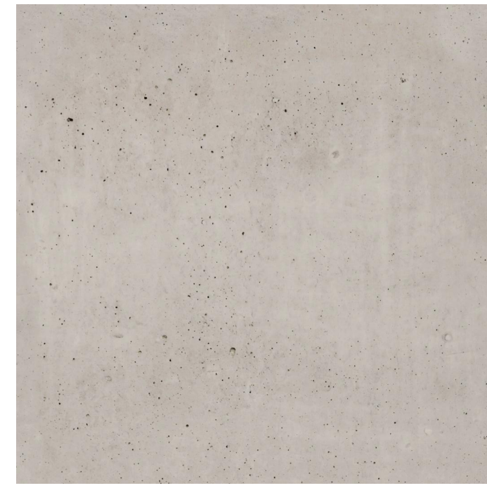
CONC NATURAL OFF-FORM CONCRETE
