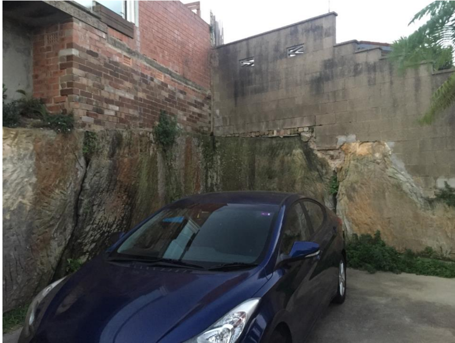
Photo 1 – Medium to high strength sandstone exposed along eastern boundary. Top of rock approximately 1m below surface level in rear garden of 48 Beacon Avenue.
