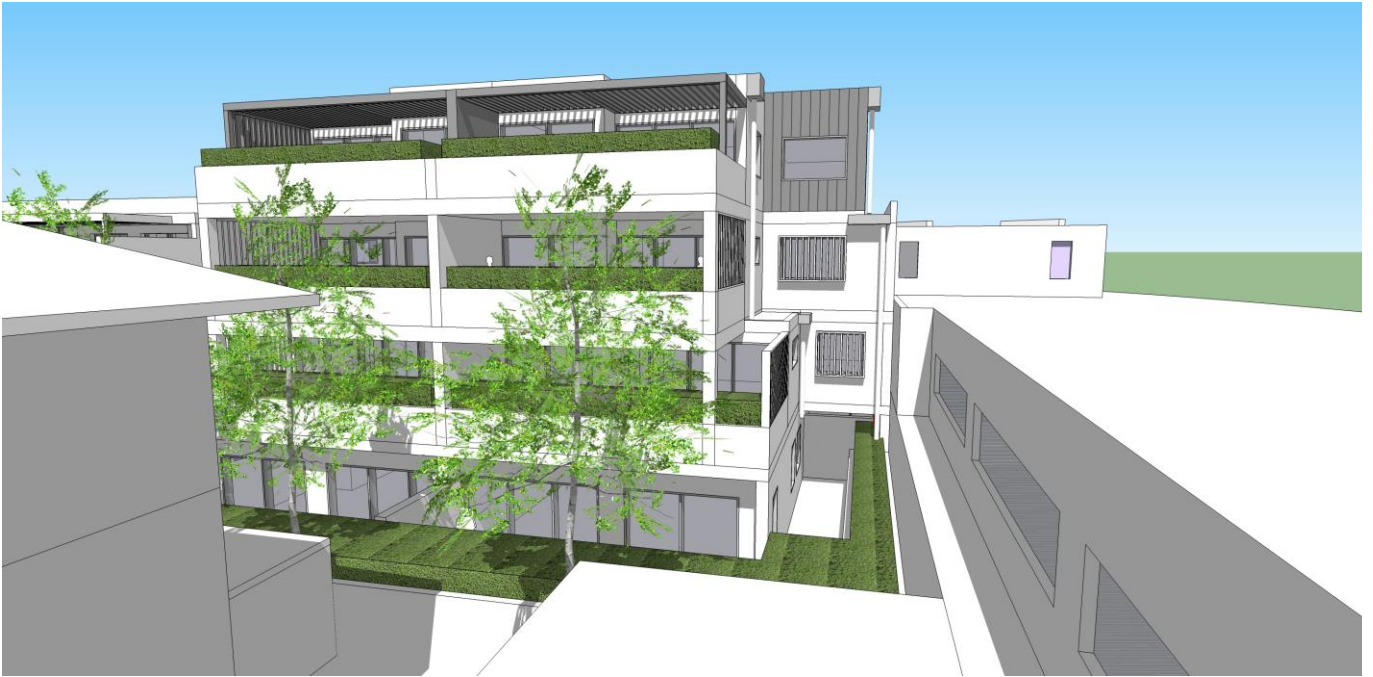
Above: Building form steps in from side and rear boundaries at the north to provide distance and privacy to residential neighbours to the north. Privacy screens fixed on balconies and north facing bedroom windows
