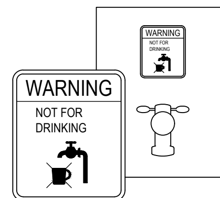
SCALE N.T.S * EVERY EXTERNAL SUPPLY OUTLET FROM RAINWATER RE-USE TANK TO BE LABELED WITH METALLIC WARNING SIGN
