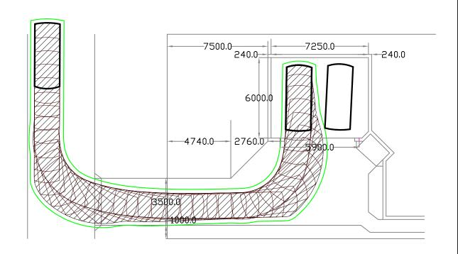
This drawing has been prepared using vehicle modelling computer software AutoTrack V5.00a in conjunction with AutoCAD 2013. The vehicle used is based upon vehicle data provided by Austroads and incorporates a reasonable degree of tolerance. However, it is not possible to account for all vehicle types/characteristics and/or driver ability.
