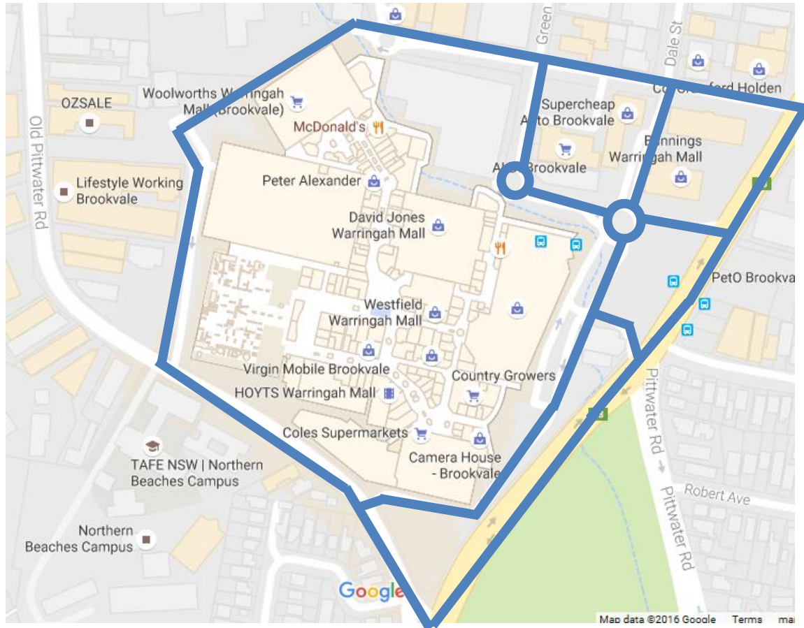
Figure 8-1: Fire Brigade perimeter vehicular access around the existing Warringah Mall building
