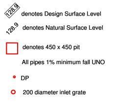
Stormwater calculations Post development impervious area = 20 sq.m. No Detention required (< 50 sq m)
