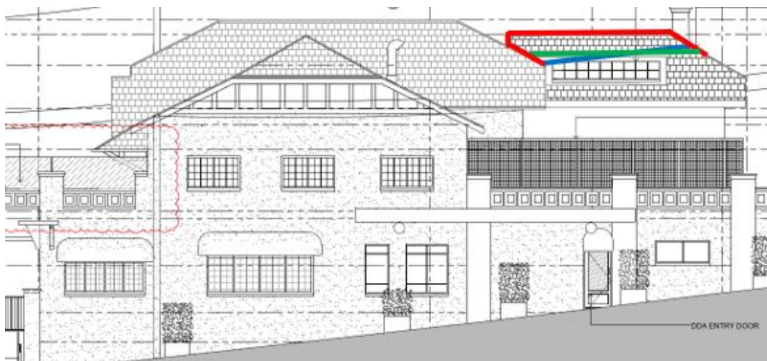
Figure 4 – Plan extract western elevation showing the height non-compliance based on ground level (existing). The blue line shows the 8.5 metre height standard, the red line the extent of proposed new works located above the height standard and the green line the existing building ridge line in this location.
