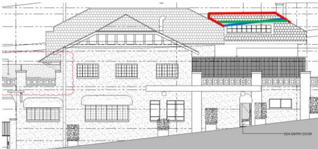
Figure 10 – Plan extract western elevation showing the height non-compliance based on ground level (existing). The blue line shows the 8.5 metre height standard, the red line the extent of proposed new works located above the height standard and the green line the existing building ridge line in this location.
