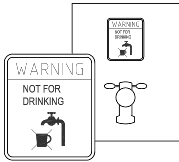
TYPICAL WARNING SIGN SCALE N.T.S * EVERY EXTERNAL SUPPLY OUTLET FROM RAINWATER RE-USE TANK TO BE LABELED WITH METALLIC WARNING SIGN
