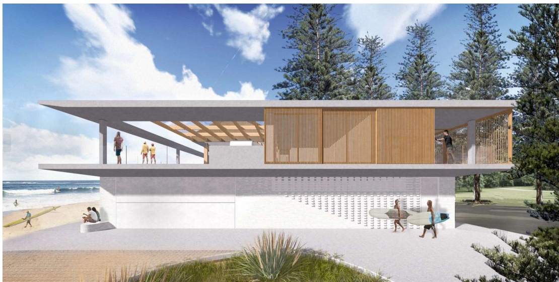
Figure 73: Northern addition designed with a streamlined, contemporary form to distinguish it from the Mediterranean style existing building. The main focus of this new portion of the building is to provide upgraded beachside access and storage for the Surf Lifesaving vehicles and equipment with an upper terrace to support the club operations and general membership. The solidity of the lower-level structure is a function of the coastal protection requirements thoughtfully integrated into the scheme. (Source: Adriano Pupilli Architect)
