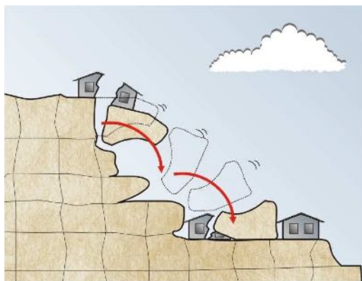
Figure 1 - Failure of an undercut block
