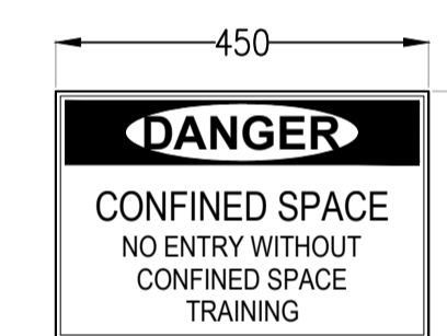
CONFINED SPACE SIGN SCALE 1:10
