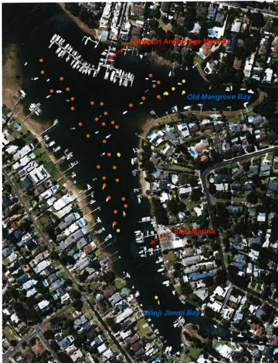
Figure 6-5: Swing moorings in locality of Sirsi Marina (orange = commercial mooring, yellow = private mooring)
