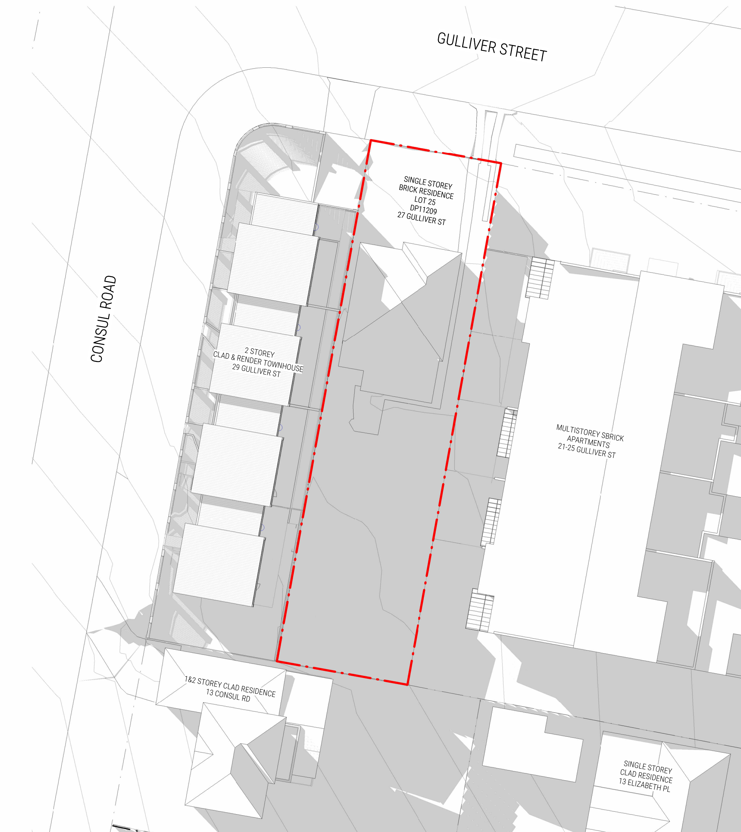
1 EXISTING SHADOW DIAGRAM - 3PM JUNE 21ST DA502/ 1:200 @ A1
