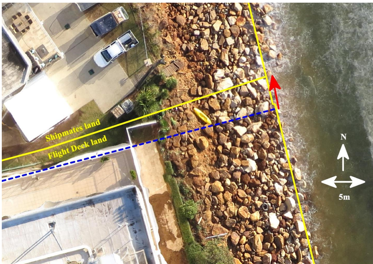
Figure 1: Alignment of northern face of Flight Deck (blue) in relation to property boundaries (yellow) and projection of proposed works north of Flight Deck building (red)
