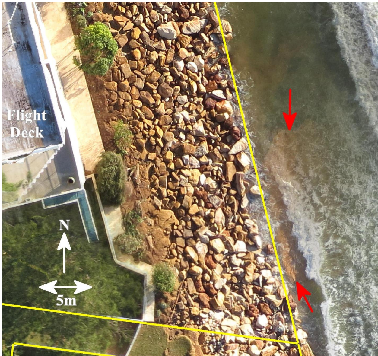
Figure 3: Cemented sand visible offshore of southern end of Flight Deck (between red arrows) on 10 June 2016
