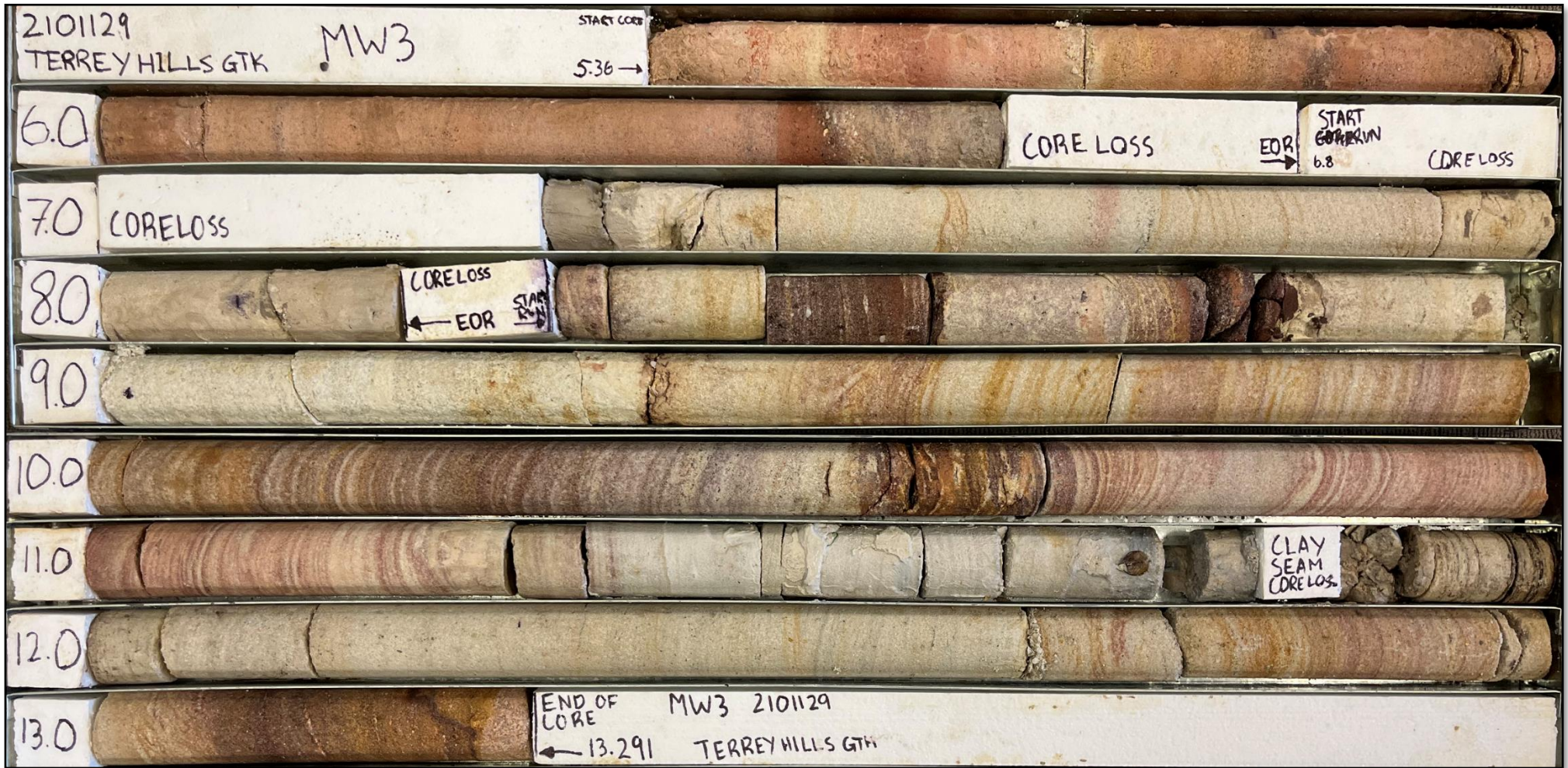
Borehole MW3 – NMLC coring completed from 5.36 to 13.29 mbg.
