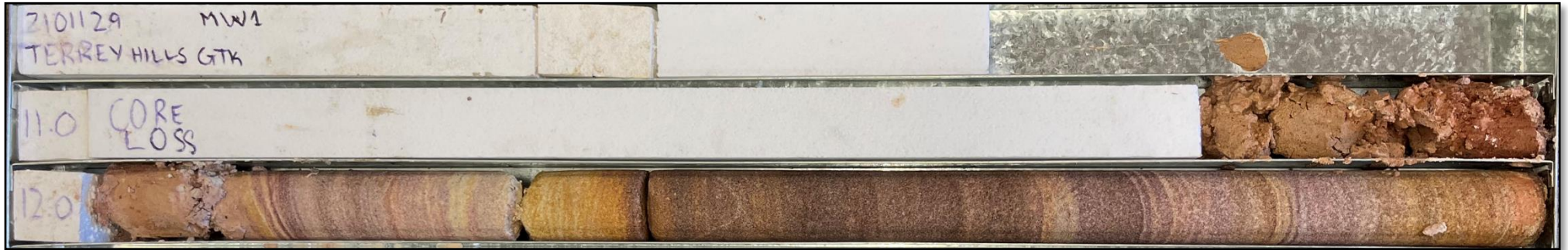
Borehole MW1 – NMLC coring completed from 11.00 to 13.00 mbg.
