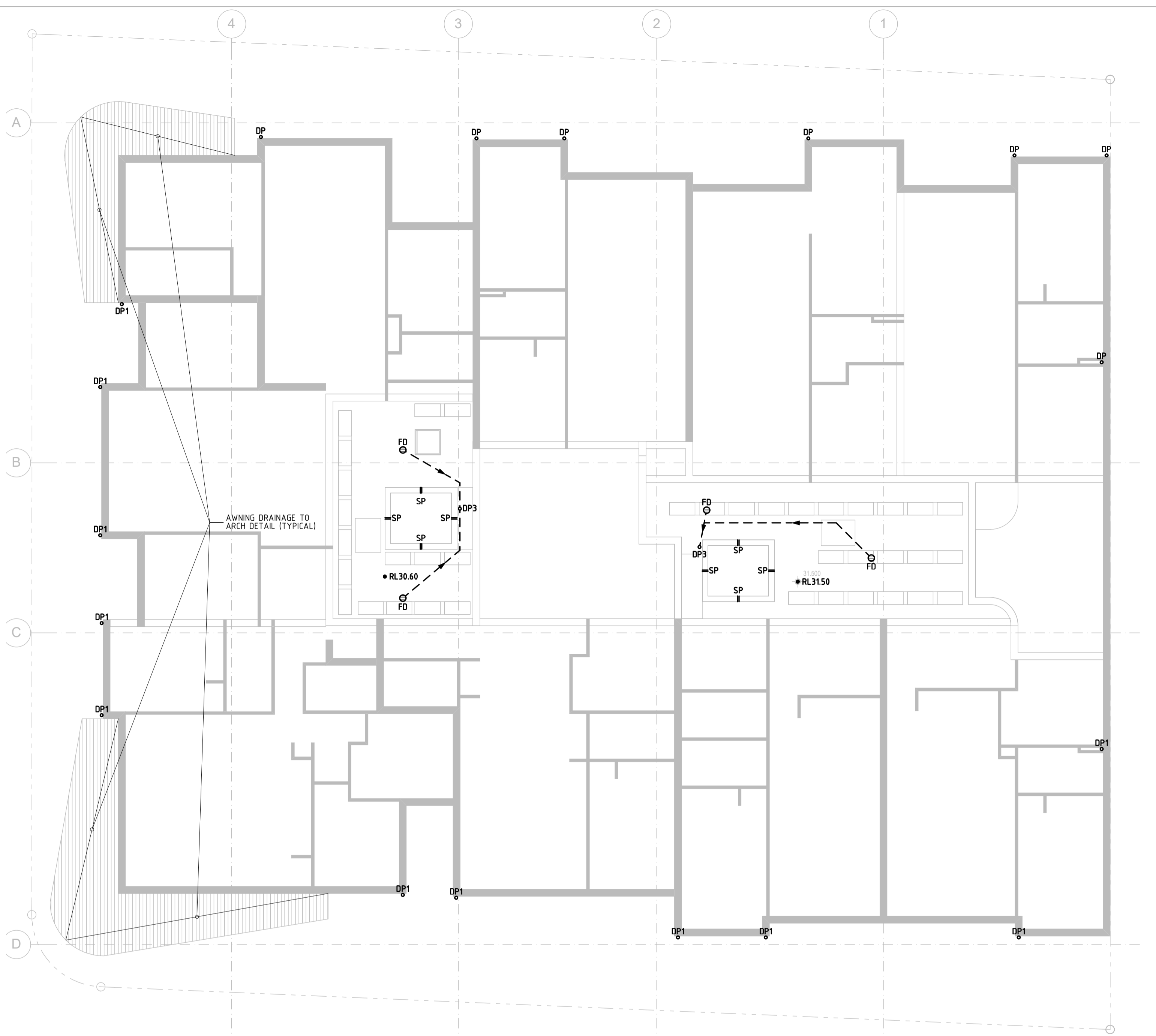
LOWER ROOF DRAINAGE PLAN
