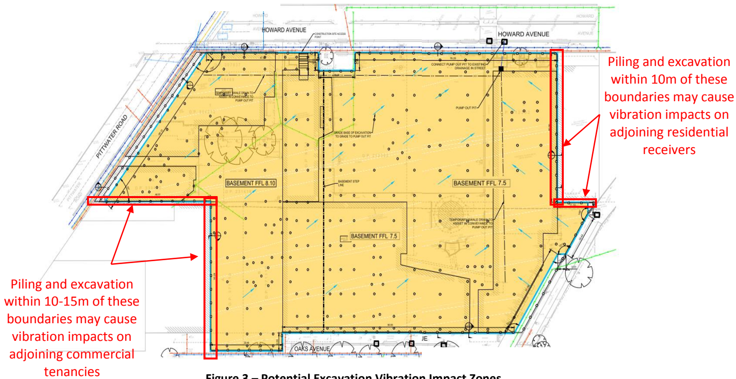
Figure 3 – Potential Excavation Vibration Impact Zones
