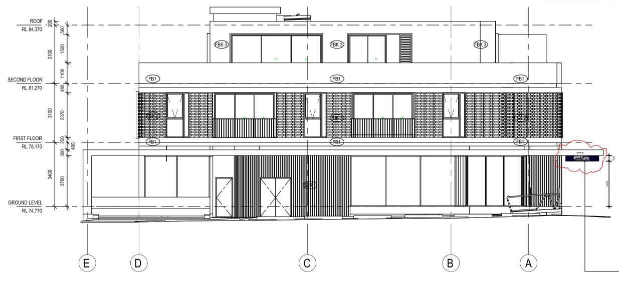
Example of illuminated under awning double sided sign box. Sign to have black anodised aluminium frame and to be fixed directly to under side of awning.
