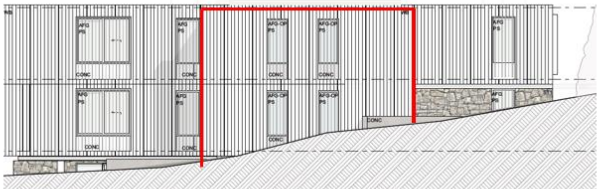
Figure 1 – Plan extracts showing portion of eastern wall setback 4 metres from eastern boundary.
