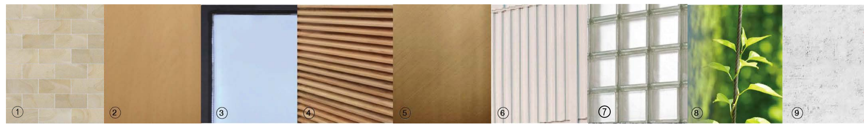
1 Sandstone cladding 2 Render in timber colour 3 Clear glazing & dark metal mullions 4 External venetian louvres 5 Render in bronze colour 6 Light coloured profiled metal 7 Glass blocks 8 Landscaped roof and ground 9 Smooth concrete 10 RSM01: Metal Roofing in Colorbond 'Shale Grey'
