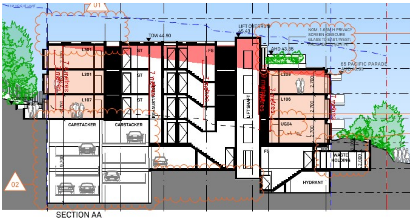
Section AA showing the side envelope breach (source Benson McCormack)
